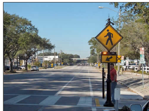
Rapid Flashing Beacon (MUTCD).
